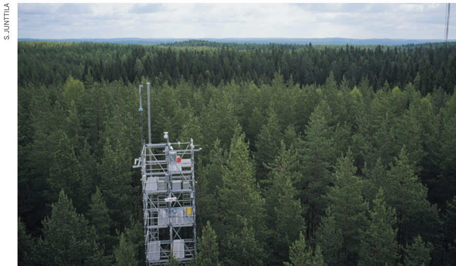
Figure 1 | Something in the air. This tower at the SMEAR II field station, Finland, supports several instruments that are used to analyse the atmosphere above the forest canopy. Mauldin et al. 1 have detected a new oxidant in the atmosphere above the station.
