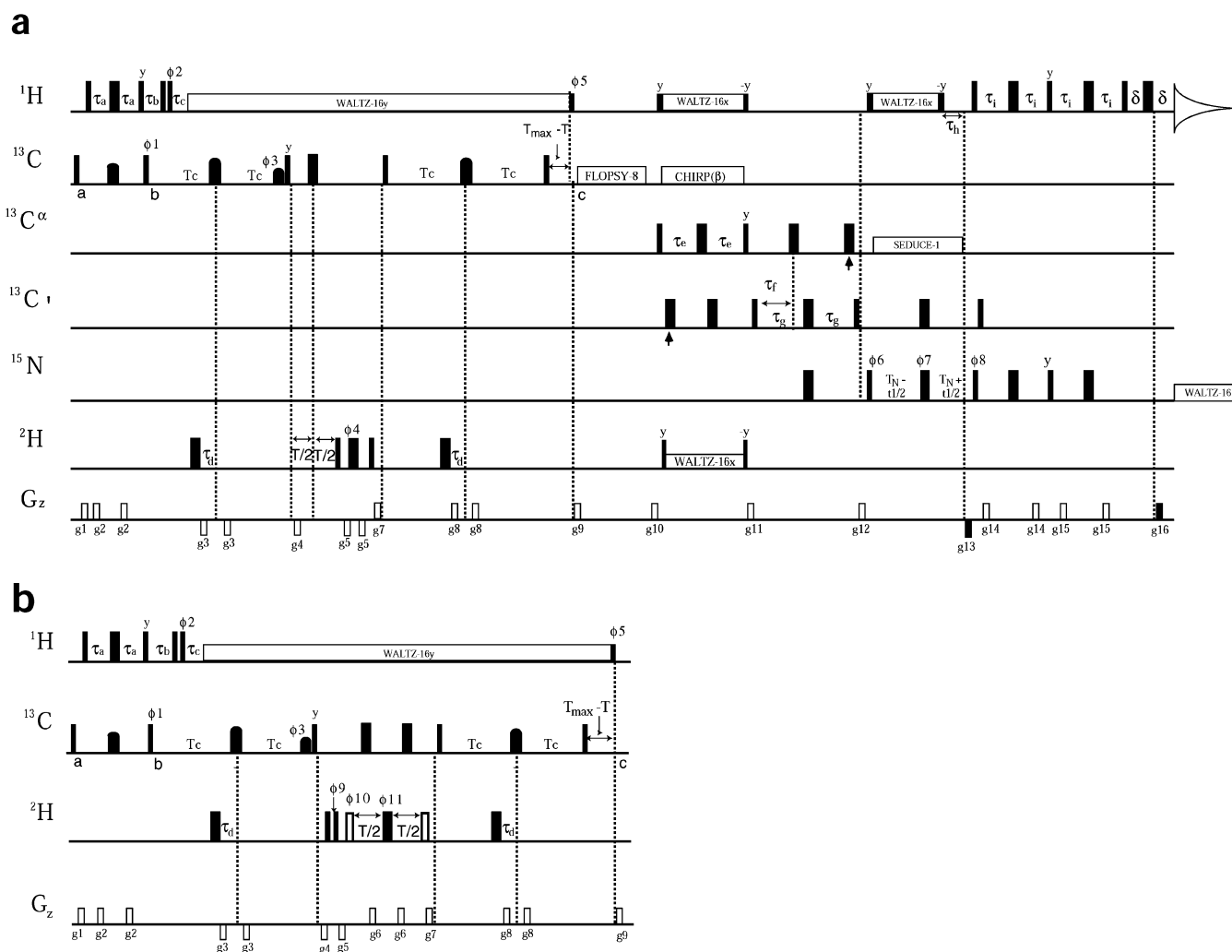
Figure 1. Pulse schemes used for the measurement of relaxation rates of deuterium quadrupolar order, 3D_z^2 - 2 , R_{3D_z^2 - 2} (a), and antiphase transverse magnetization, D_z D_z + D_z D_z , R_{D_z D_z + D_z D_z} (b), in unfolded protein states. Similar pulse schemes for the measurement of R_{D_z} and R_{D_\alpha} in unfolded proteins have been described previously 19 (minor modifications that have recently been incorporated are available from the authors upon request). All narrow (wide) rectangular pulses correspond to flip angles of 90^\circ ( 180^\circ ) and are applied along the x -axis, unless otherwise indicated. Carriers are positioned at the water frequency ( ^1\text{H} ), 119 ppm ( ^{15}\text{N} ), 0.8 ppm ( ^2\text{H} , start of sequence until the end of the FLOPSY 65 mixing scheme), 4.7 ppm ( ^2\text{H} , immediately after FLOPSY mixing until the end of the sequence), 20 ppm ( ^{13}\text{C} , start of sequence until FLOPSY-8), 43 ppm ( ^{13}\text{C} FLOPSY mixing), and 58 ppm ( ^{13}\text{C} , immediately after the FLOPSY-8 until the end of the sequence). All proton pulses are applied with a 32.5 kHz field, with the exception of the 6.4 kHz field used for WALTZ decoupling 66 and the pulses immediately flanking the decoupling elements (also 6.4 kHz). The ^{13}\text{C} shaped 180^\circ pulses between points a and b (1.36 ms at 600 MHz, centered at 19.5 ppm) and in the middle of the 2T_c periods (392 \mu\text{s} , 41 ppm) have RE-BURP profiles. 67 The ^{13}\text{C} pulse of phase \phi_3 (640 \mu\text{s} , centered at 57 ppm) is applied with the SEDUCE-1 shape. 68 Magnetization relay through TOCSY mixing is achieved using the FLOPSY-8 scheme (8 kHz field, 7 cycles). ^{13}\text{C}_\beta decoupling fields, centered at both 29.5 ppm ( \pm 14.5 ppm) and 70.0 ppm ( \pm 2 ppm) and denoted by CHIRP( \beta ), were implemented using a scheme comprised of 5 ms WURST-2 pulses. 69 The decoupling element was created using the Varian tool Pbox. All ^{13}\text{C}_\alpha rectangular pulses have durations which minimize excitation in the carbonyl region of the carbon spectrum and vice-versa. 70 Pulses indicated with vertical arrows are used to compensate for Bloch–Siegert effects. 71 ^{13}\text{C}_\alpha WALTZ decoupling during the constant time 2T_N period was achieved with 326 \mu\text{s} SEDUCE-1 pulses centered at 58 ppm. All ^{15}\text{N} pulses are applied with a 5.8 kHz field, with 1.1 kHz WALTZ-16 decoupling during acquisition. ^2\text{H} WALTZ decoupling employed a 0.7 kHz field; all other ^2\text{H} pulses are 2.0 kHz. The narrow rectangular pulses that are not filled in part b have flip angles of 45^\circ . The delays employed are as follows: \tau_a = 1.7 ms, \tau_b = 3.85 ms, \tau_c = 1.93 ms, T_c = 14.5 ms, \tau_d = 1.7 ms, \tau_e = 4 ms, \tau_f = 4.4 ms, \tau_g = 13.0 ms, \tau_h = 5.5 ms, \tau_i = 2.4 ms, T_N = 15 ms, and \delta = 0.5 ms. T_{\text{max}} is chosen equal to the maximum value of T (relaxation delay) that is used in the relaxation series. The phase cycling is as follows: \phi_1 = 2(x) , 2(-x) ; \phi_2 = x , -x ; \phi_3 = 4(x) , 4(-x) ; \phi_4 = 4(0^\circ) , 4(45^\circ) , 4(90^\circ) , 4(135^\circ) ; \phi_5 = -x , x ; \phi_6 = 16(x) , 16(-x) ; \phi_7 = 2(x) , 2(-x) ; \phi_8 = x ; \phi_9 = 4(x) , 4(-x) ; \phi_{10} = 8(x) , 8(-x) ; \phi_{11} = 16(x) , 16(-x) . For part a, rec. = x , 2(-x) , x , -x , 2(x) , -x , x , 2(-x) , x , -x , 2(x) , -x . After 16 scans, the phase of the receiver is inverted. For part b, rec. = x , 2(-x) , 2(x) , 2(-x) , x , -x , 2(x) , 2(-x) , 2(x) , -x . After 16 scans, the phase of the receiver is inverted. The durations and strengths of the gradients are g_1 = (0.5 ms, 5 G/cm), g_2 = (0.3 ms, 3 G/cm), g_3 = (0.3 ms, -25 G/cm), g_4 = (0.2 ms, -10 G/cm), g_5 = (0.4 ms, -10 G/cm), g_6 = (0.05 ms, 25 G/cm), g_7 = (0.25 ms, 6 G/cm), g_8 = (0.2 ms, 10 G/cm), g_9 = (0.6 ms, 15 G/cm), g_{10} = (1.0 ms, 15 G/cm), g_{11} = (0.4 ms, 6 G/cm), g_{12} = (0.5 ms, 25 G/cm), g_{13} = (1.25 ms, -30 G/cm), g_{14} = (0.2 ms, 2.5 G/cm), g_{15} = (0.3 ms, 2.0 G/cm), and g_{16} = (0.125 ms, 29.6 G/cm). Quadrature detection is achieved in t_1 using the enhanced sensitivity gradient approach, 72,73 with separate FIDs recorded for each t_1 point corresponding to ( \phi_8 = x , g_{13} ) and ( \phi_8 = -x , -g_{13} ). Decoupling is interrupted prior to the application of gradients. 74
